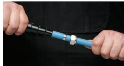
2. Slide nut and split ring over pipe and bevel the inside of the pipe by inserting then rotating the beveling tool.
